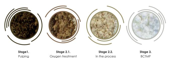
Getting bleached chemi-thermomechanical pulp includes steaming chips, grinding in two stages with its chemical treatment and bleaching.
