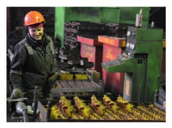
The core sections of the workshop provide the production of sand cores by rapid tooling, both during heating and in the Hardening Tar-Sand Process.
