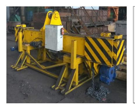
manipulator The allows lowering mechanism and raising the half-molds precisely positioning them at the place of assembly of the molds as the operator works "from the ground". The use of the manipulator on a radio control reduced the percentage of rejects and improved working conditions in increased labor general: productivity, personnel safety.
